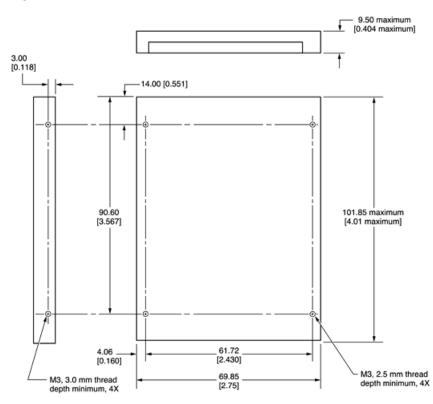
Figure 3-4 Maximum dimensions of the internal hard disk
